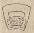
economised, and the temperature of the crucible increased, by using a jacket like that represented partly in section and partly in perspective in the wood cut. It is to be made of sheet copper or iron, open at the top and bottom, and within it, three projecting slips of iron-plate are to be fixed by rivets, intended to support
